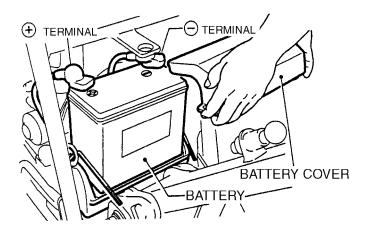
Figure 29. Battery Maintenance
